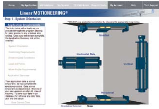
Your System Mounting Orientation is stored in the database to allow bearing and ball screw safety factor calculations.
