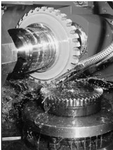
CNC machining of a PowerTRUE right-angle gear
